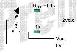
Typical installation: Customer has to select suitable resistors for their chosen supply voltage. Forward voltage of LED is 1.3V and LED current should be 10mA (depending on application liquid). Therefore, for a supply of Vs:
